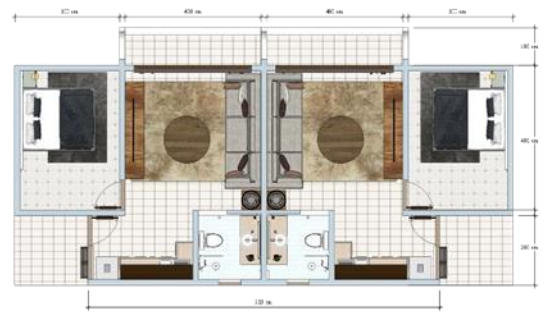
Gambar 16. Denah unit kamar
